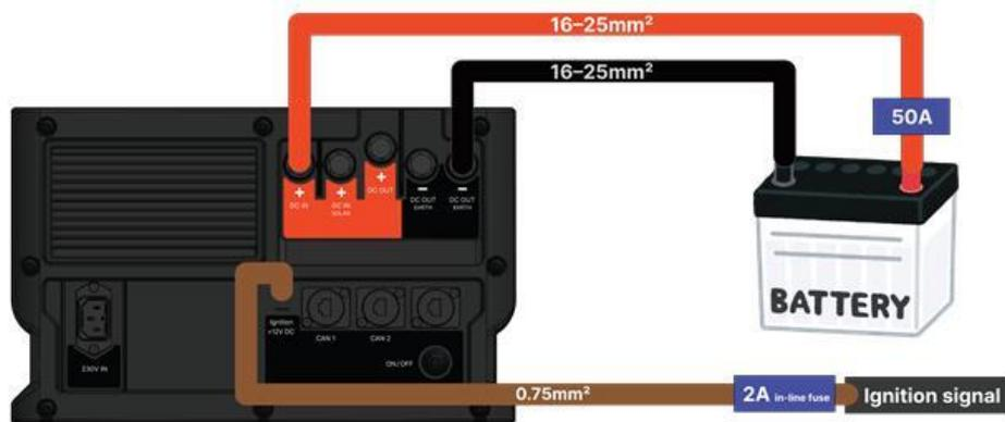
Figure 2 DC Charging for non-electrical vehicles
