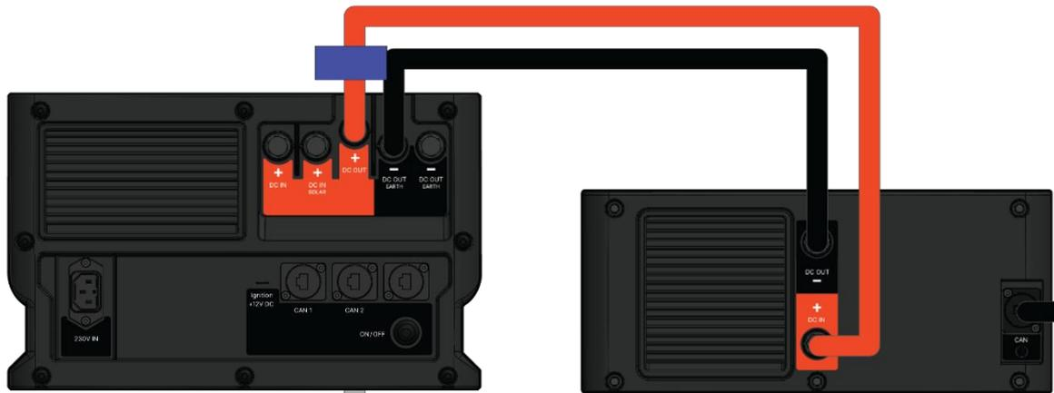
The e-Inverter and e-Heater should be wired to the positive and negative DC IN on the rear of the e-Power.
