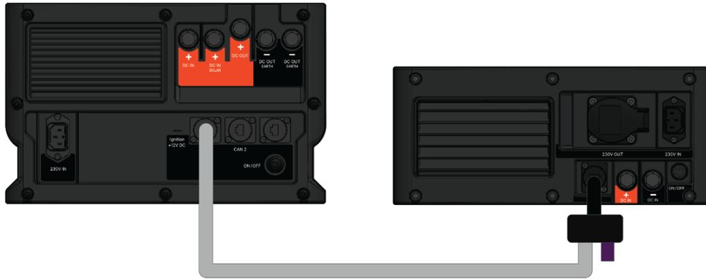
Figure 3 RJ45 cable between the e-Power and e-Inverter with termination at the end
